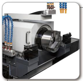
With high rigidity A2-6 taper spindle. This spindle provides excellent radial rigidity, stable thermal, minimum heat deformation, and high dynamic accuracy to guarantee absolutely grinding quality.
