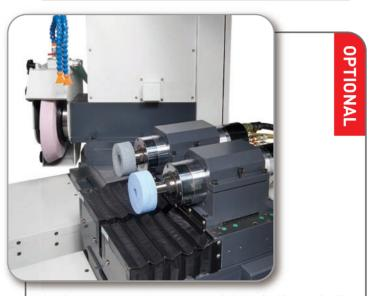
Y axis applys to sleeve type rigid grinding spindle with Ø405mm grinding wheel (wheel angle 25°) Z axis applys to BUILT-IN type grinding spindle Z2 axis applys to BUILT-IN type grinding spindle
